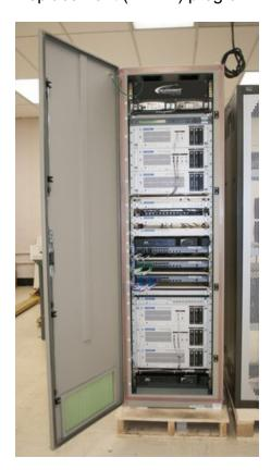
Telephonics developed the CTD system to process and convert radar signals from the legacy ASR-8 and Beacon ATC radar systems to the latest digital data standards required by STARS, which are being installed throughout the U.S.
