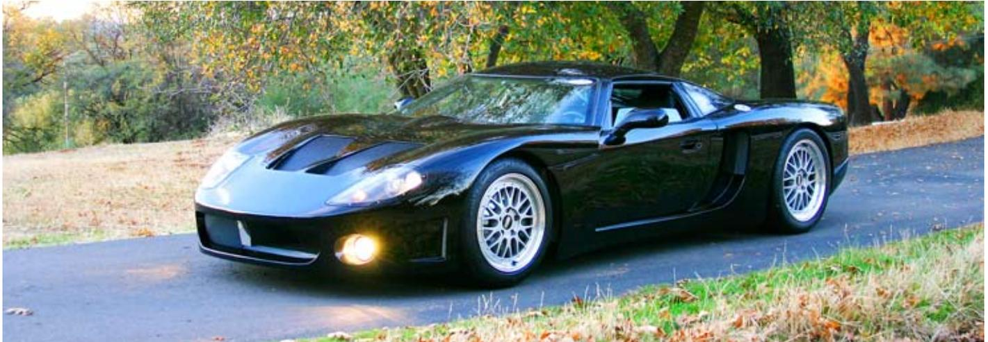
The Capstone CT-380 hybrid, based on a Factory Five sports car chassis, uses a 30 kw/40 hp turbine engine to provide power to charge its Li-ion battery pack.
