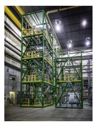
This 25 meter-tall unit will confirm the viability and suitability of the Bio-TCat process for scale-up, and generate the data needed to design commercial plants using Bio-TCat
