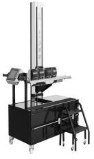
The L-300 system (at left), the latest addition to Amtech's automation line, was designed for fabrication houses with older diffusion equipment where a load station is not used. This system allows basic automation to be used on equipment that was entirely manually loaded in the past.
