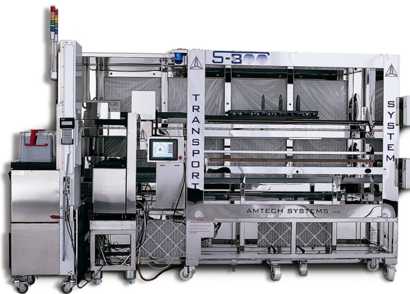
(Above) The products described above and on the preceding page are highly complementary and synergistic. They are sold to the same customers, through the same distribution channels, often as fully integrated systems. Above is an Amtech loadstation (background), S-300 automation system (right of center), a third-party SMIF pod cassette on a SMIF pod opener and wafer transfer machine (far left).
