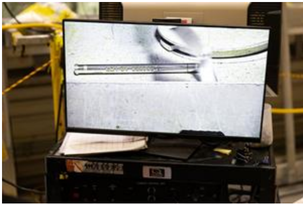
Image 3: A capsule with an irradiated Lightbridge coupon sample inside after removal from the ATR (May 6, 2026)
