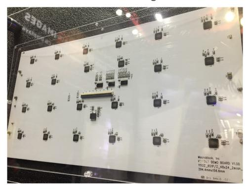
PCB based - 1152 LEDs (each of the 24 ICs is wired to 48 LEDs) - for several 000's of zones this becomes too costly
