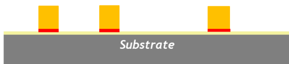
Step2: Coating smartkem ILD (negative-type ILD)
