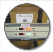
Utilizes light indicators to help increase the speed, accuracy and efficiency of material handling tasks
