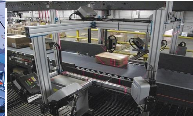
Multiple integrated distribution and fulfillment systems (including laser-based identification and dimensioning technologies) communicate in a warehouse to identify and route items and parcels through the facility and out to a customer.
