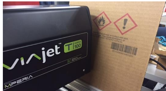
Non-contact ink-jet printing units apply print on products.
