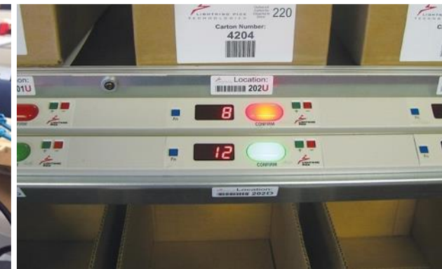
Industrial's Pick-to-Light Systems utilizing light indicators for sorting and control of merchandise.
