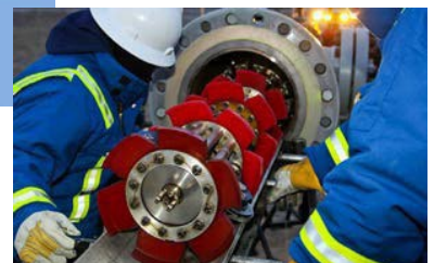
Pipelines deliver massive amounts of crude daily and ensuring safe operation is key. The EMCORE TAC-450-DSP1750, coupled to additional sensors, provides these inspection robots with extremely accurate angular data.
