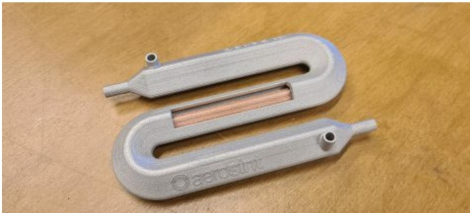
This multi-metal heat exchanger is printed using Aerosint selective powder deposition technology with stainless steel exterior surfaces to match other components in a cooling circuit and copper alloy interior surfaces for improved corrosion resistance. (Photo: Business Wire)
