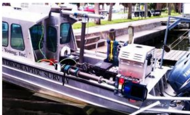
Figure 1: George F Young preparing to survey structures with the Echoscope
