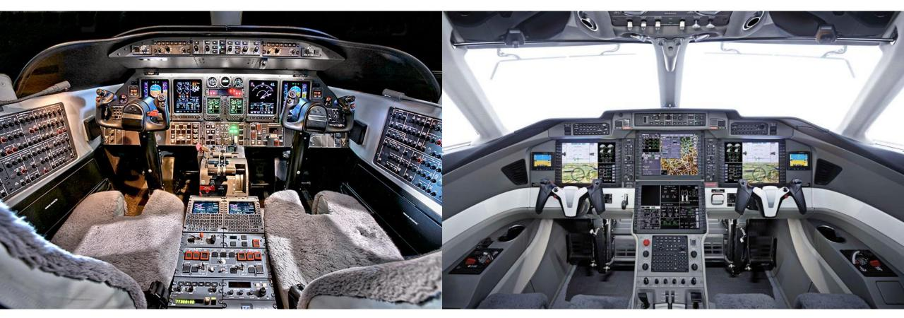
Traditional Cockpit with Circuit Breakers Learjet 45 Electronic Power Distribution PC-24
