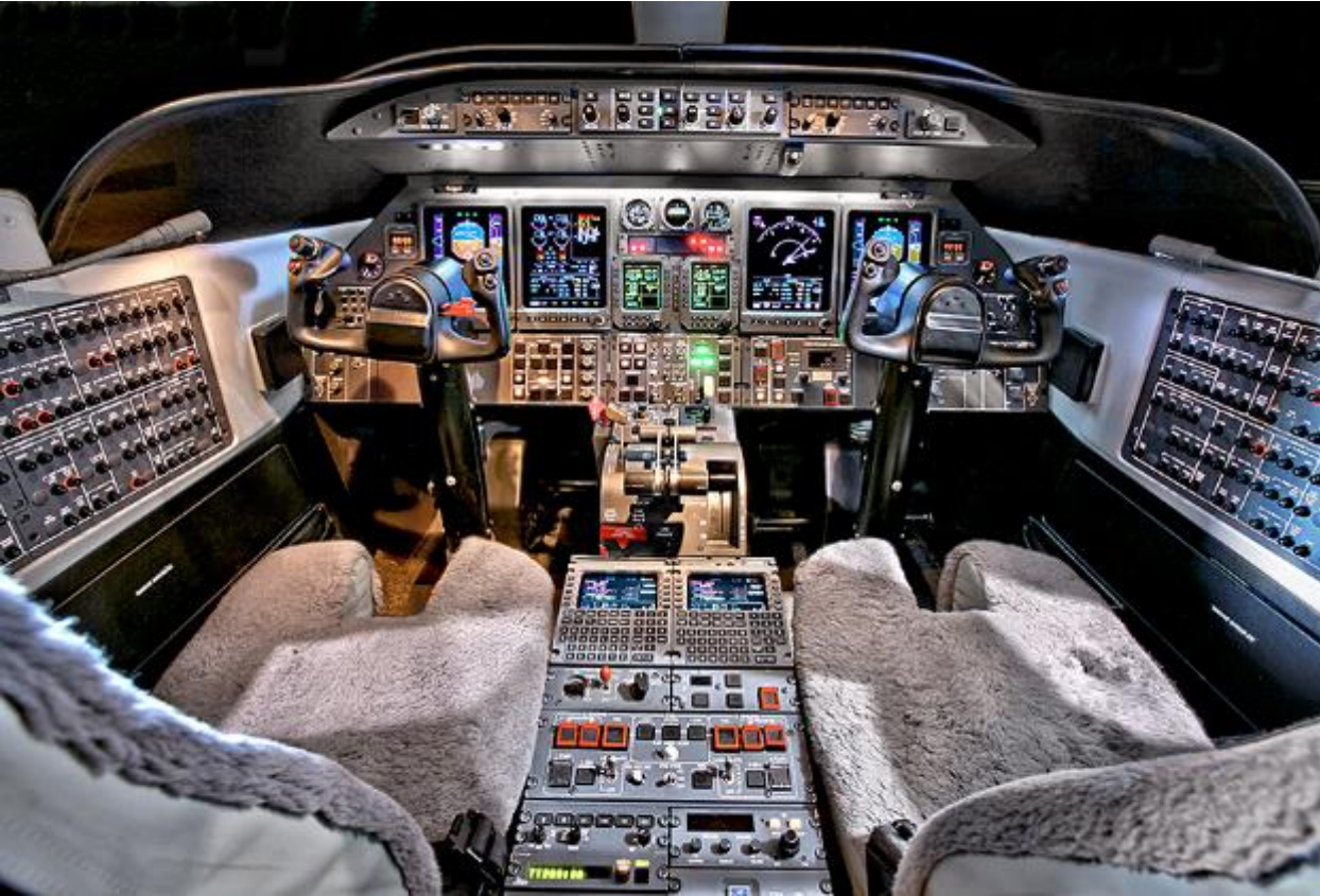
Traditional Cockpit with Mechanical Circuit Breakers Learjet 45
