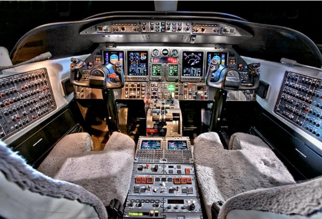
Traditional Cockpit with Circuit Breakers Learjet 45
