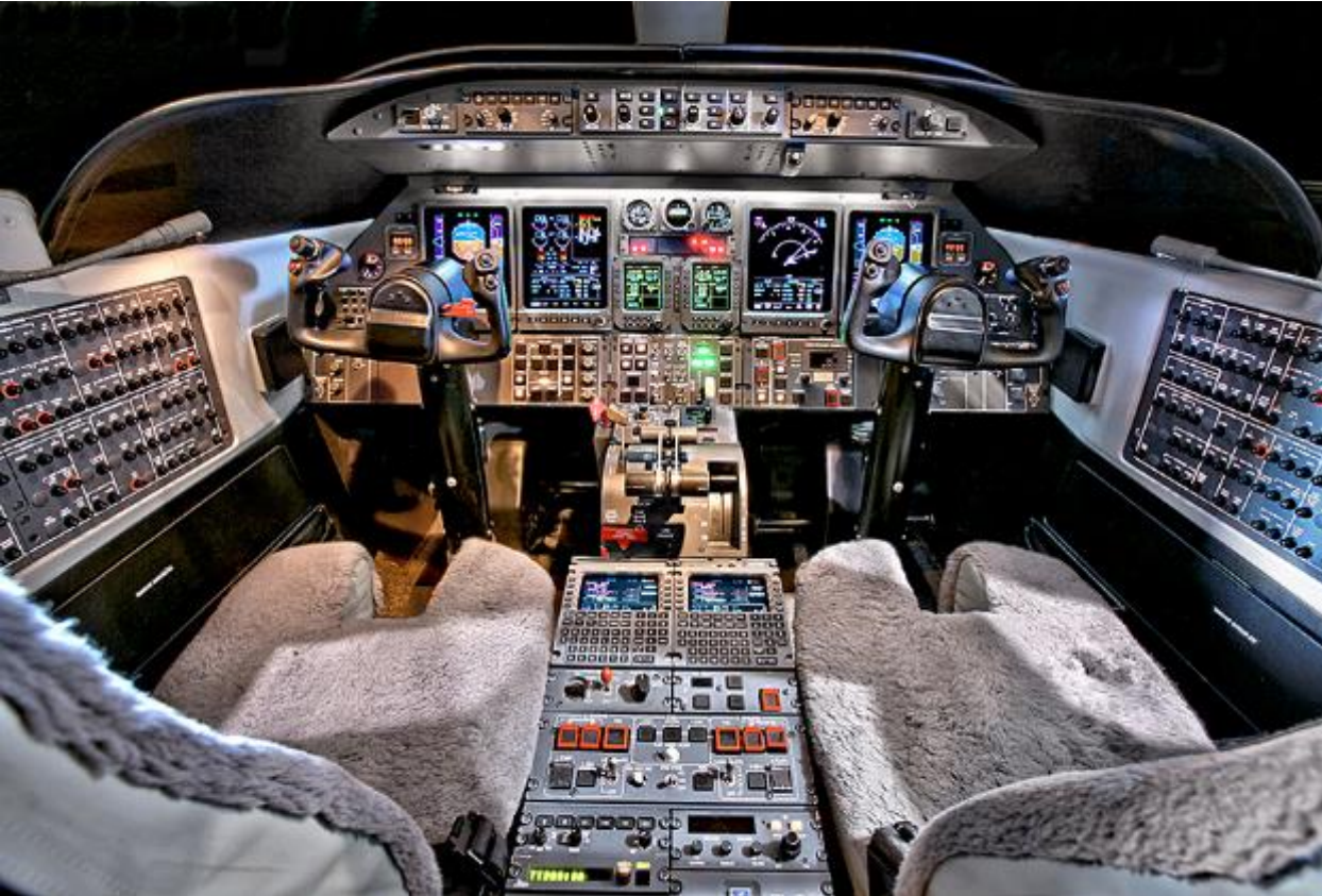
Traditional Cockpit with Circuit Breakers Learjet 45
