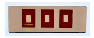
**PV Nano Cell: Printed Capacitors**
