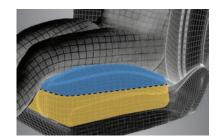
Some premium seat manufacturing uses two pieces of foam or a 'topper' with pad adhered together. The bottom piece of foam is firm while the top piece of foam is soft. The result is added steps and cost in the manufacturing process.
