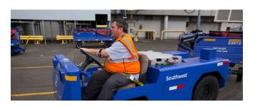
This baggage tug is a new electric vehicle that is part of our initiative to modernize our GSE fleet, making it more efficient and reliable by running on electricity instead of traditional gasoline or diesel fuel.
