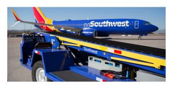
Our Ramp Agents appreciate that electric GSE, such as this belt loader, are quieter and cleaner than gasoline or diesel-powered machines.
