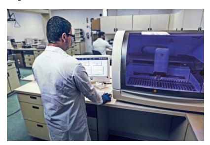
Laboratorians and clinicians can use the BD MAX™ MDR-TB Assay to simultaneously detect bacteria that cause tuberculosis (TB) and determine if the bacteria contain mutations associated with resistance to two important first-line drugs, isoniazid (INH) and rifampicin (RIF), enhancing the information available to direct the optimal treatment for their patients.
