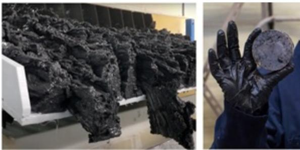
Ultrapure spongy metal from the AquaRefining electrolyzers are then compressed into briquettes which the Company believes can now go directly to new battery manufacturing.
