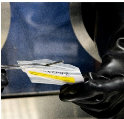
A close-up view of a finished enriched uranium-zirconium coupon sample
