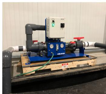
Moleaer's nanobubble generator is easy to install, rapidly integrating with existing tanks and irrigation systems to boost dissolved oxygen levels in feed water.
