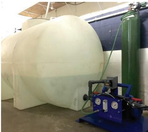
*Moleaer's nanobubble generator saturates the feeder tank with nanobubbles before being dispersed into the irrigation system.*
