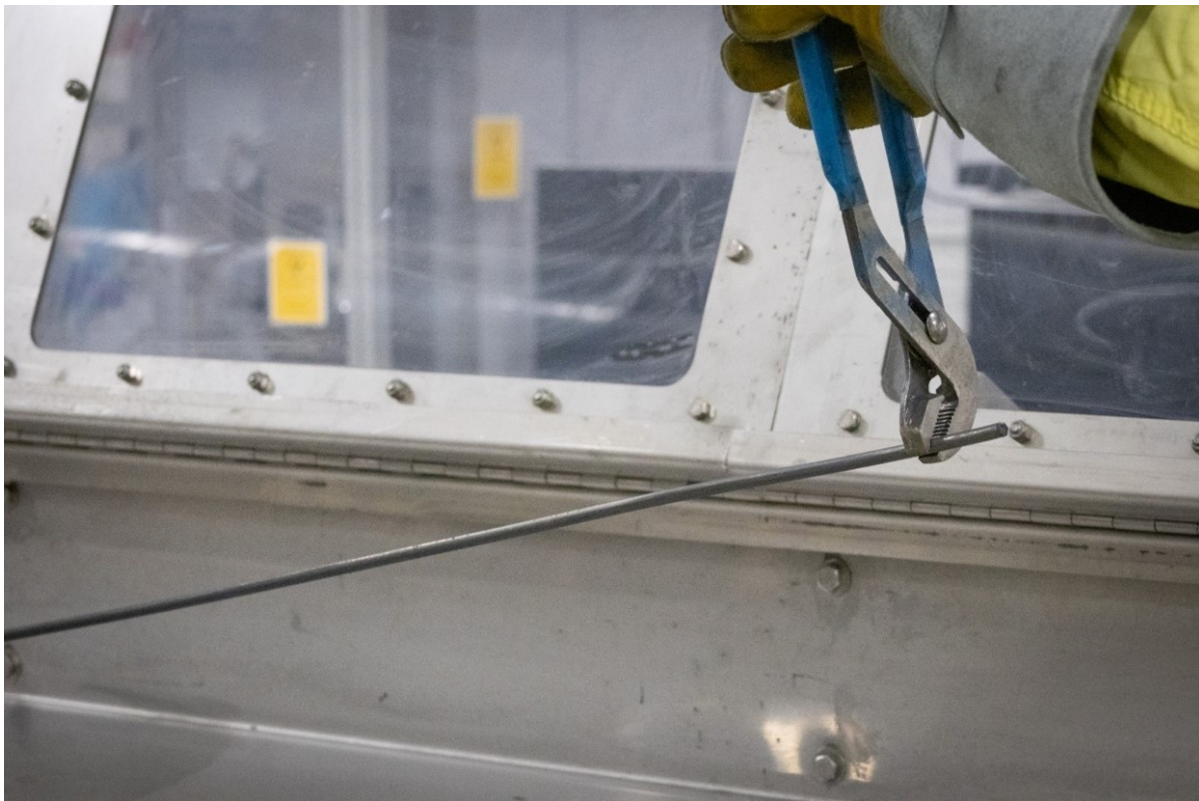
Figure 3: Co-extruded rod sample after co-extrusion process
