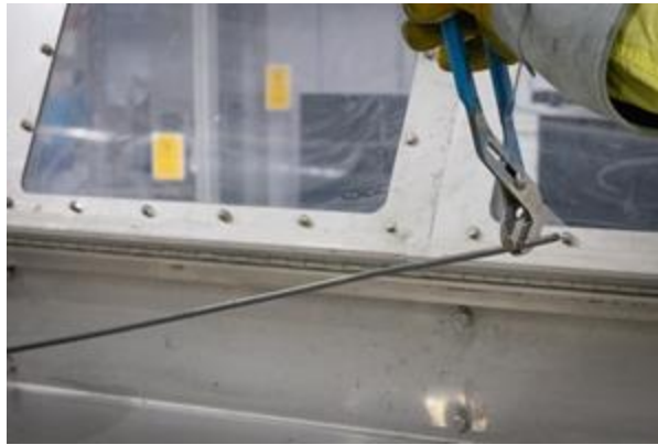
Co-extruded rod sample after co-extrusion process
