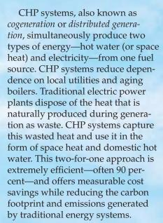
According to the U.S. Environmental Protection Agency, "By capturing and utilizing heat that would otherwise be wasted from the production of electricity, CHP systems require less fuel than equivalent separate heat and power systems to produce the same amount of energy. Because less fuel is combusted, greenhouse gas emissions, such as carbon dioxide (CO²), as well as criteria air pollutants like nitrogen oxides (NOx) and sulfur dioxide (SO²), are reduced" (epa.gov/chp/basic/environmental.html).
