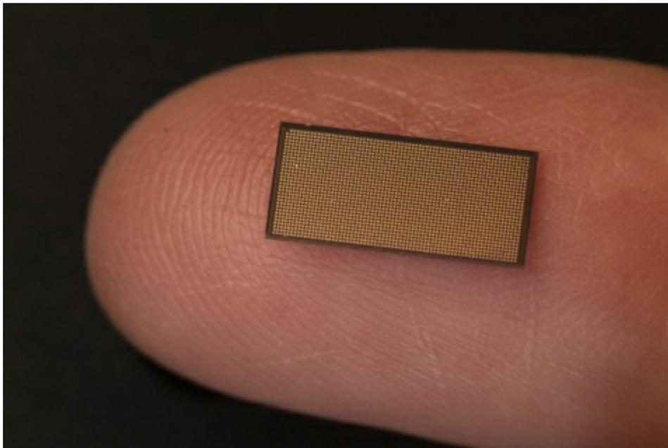
A photo shows Intel's Loihi 2 neuromorphic chip on the tip of a finger. Loihi 2 is Intel's second-generation neuromorphic research chip. It supports new classes of neuro-inspired algorithms and applications, while providing faster processing, greater resource density and improved energy efficiency. It was introduced by Intel in September 2021. (Credit: Walden Kirsch/Intel)
