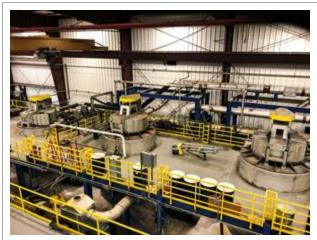
An additional kettle (far left) has been installed to process the metallic lead from the batteries we break. Ingots casted from this kettle will initially provide up to 25% increase in ingot production thus increasing revenue beyond what we receive now for selling the metallic lead as scrap metal. This is another step in bringing us closer to achieving positive contribution margin.
