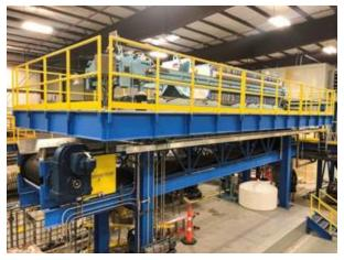
The membrane filter press has been a complex installation (concrete footing, steel structures, electrical, plumbing and controls) and is currently going through the commissioning process. We expect this piece of equipment to have a positive impact on throughput and contribution margin when it is fully operational in late Q1 by bringing us from the 67%, already achieved, to 75% of our electrolyte recovery goal.
