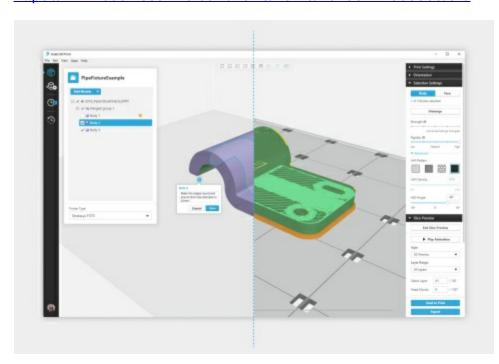
GrabCAD Advanced FDM eliminates the CAD-to-STL conversion process - creating new possibilities for designers and engineers with 3D Printing. (Graphic: Business Wire)
