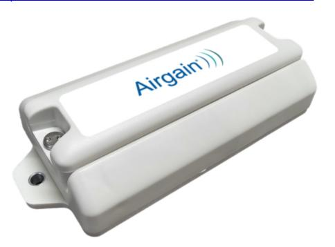
Airgain has released its AT-Flight asset tracker for real-time tracking across ground and air transportation. (Photo: Airgain)
